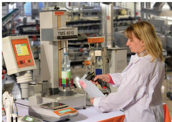
▲ Steinfurth’s compact package analyzer is a customized modular extendable mini lab that can be installed and operated directly on the bottling line. (Image courtesy of Steinfurth Inc.)
