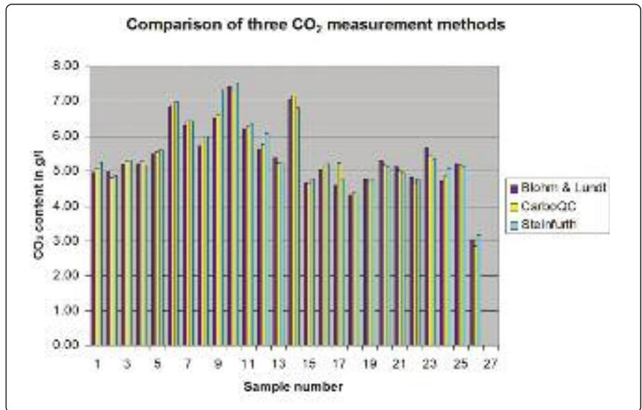
Comparison of Blohm & Lundt's method with the Steinfurth tumbling method and Carbo QC.
